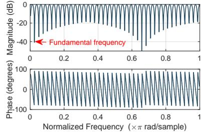
Fig. 11. Response of adaptive comb notch filter.
