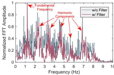
Fig. 10. Spectrum of the output of differentiator.
