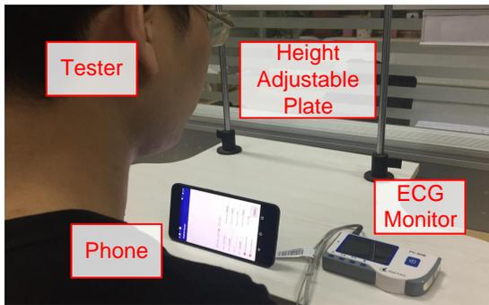
Fig. 13. Experiment setup.
